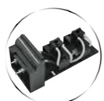
Water is circulated through this cell holder to maintain the sample cell at a constant temperature.
