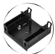
Suitable for low concentration or low absorbance samples. (Path length : 10 mm, 20 mm, 30 mm, 40 mm, 50 mm and 100mm).
